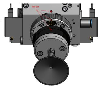
After inserting gently press tool into base and turn coupling ring.
