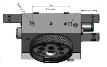
If a pneumatic gripper is mounted the two valves actuate the gripper in its two directions. Feedback is achieved via the grippers standard 2 (or 3) position sensors. Both external and internal gripping is possible.
