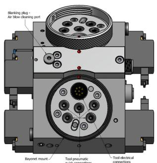
The toolbase utilizes two pneumatic valves for each of the two tool positions. Via the patented configuration which is built into the connection between the tool and the base the same two valves can be used to control pneumatic grippers or suction grippers.
