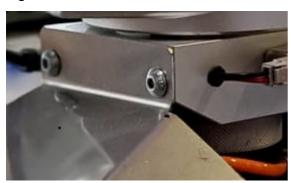
Mount the jaws on the M8 threads secure with the supplied thumb nuts.
